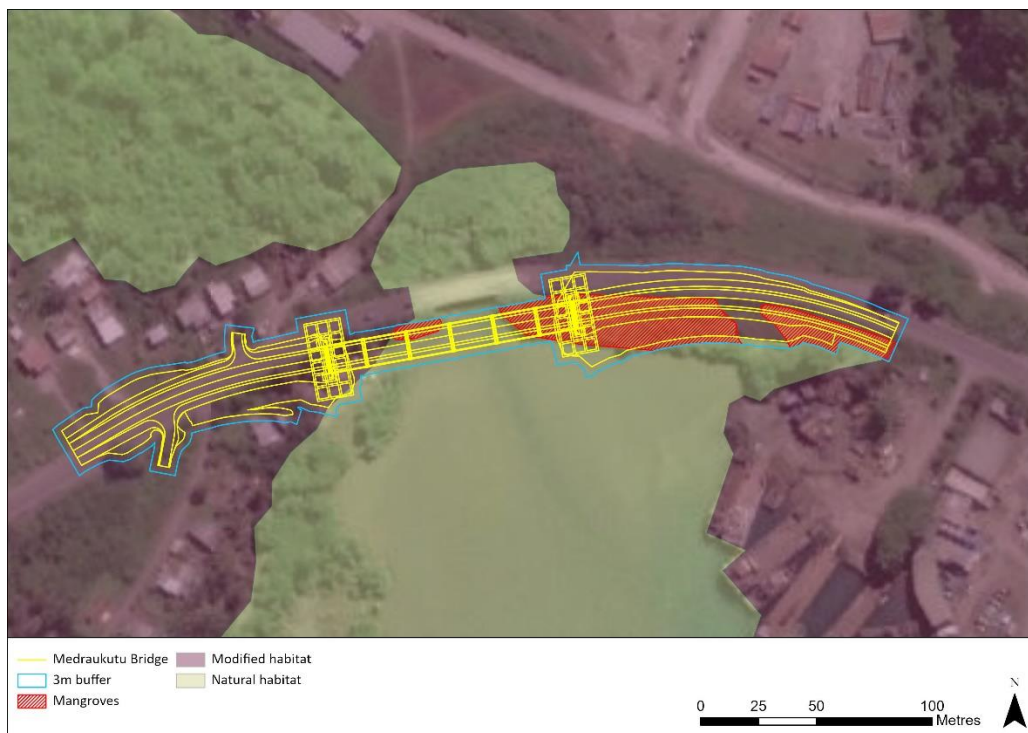
Figure 6. The natural and modified habitat surrounding the proposed bridge site.
