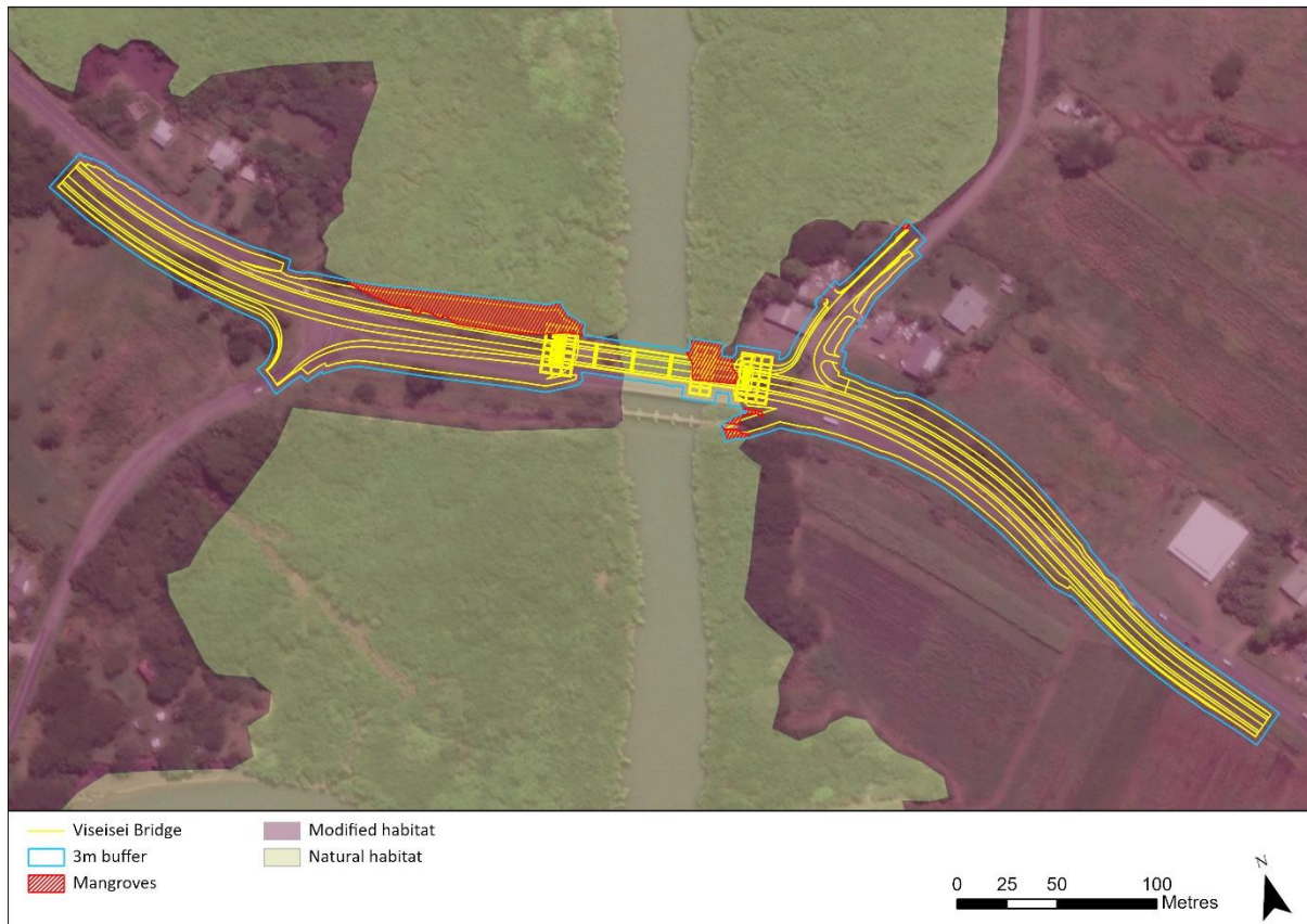
Figure 9. The proposed bridge design and area of mangroves which will be potentially removed includes a 3-meter buffer impact zone and the surrounding modified and natural habitat.
