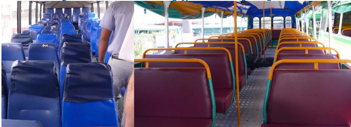
Figure 3 Bus interiors illustrating typical 3-2 seating configuration
