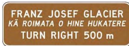
FIGURE 1.13: A TYPICAL DUAL NAME TS-2 TYPE (Secondary name is longer than the primary name)
