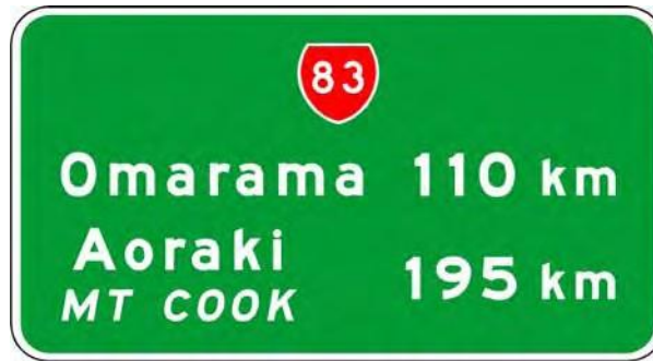
FIGURE 1.9: A TYPICAL DUAL NAME CD-1 TYPE CONFIRMATION DIRECTION SIGN (Secondary name longer than primary name)
