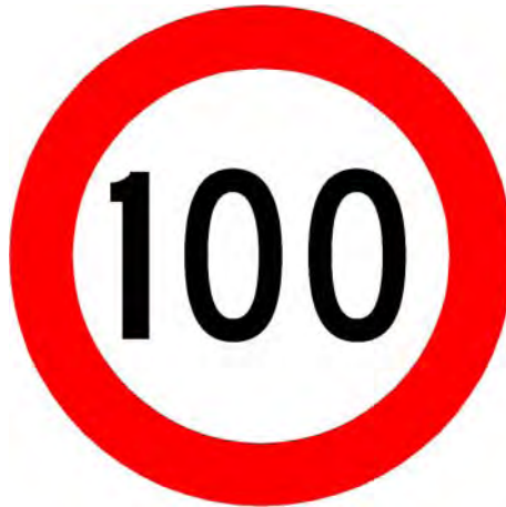
RG - 2 LEGEND : black BACKGROUND : reflectorised white BORDER : reflectorised red
