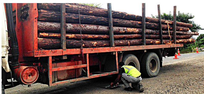
An LTA Officer uses the portable weighbridge that shows that this logging truck is loaded within the legal limits.
